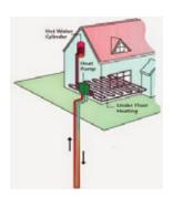
Geothermal Radial Drilling - A relatively new system which allows for sustainable heat extraction from a wider ground source is the Geothermal Radial Drilling system. Radial drilling draws its heat by spacing bores at varying angles ensuring that the highest possible ratio of watts per metre is achieved.
